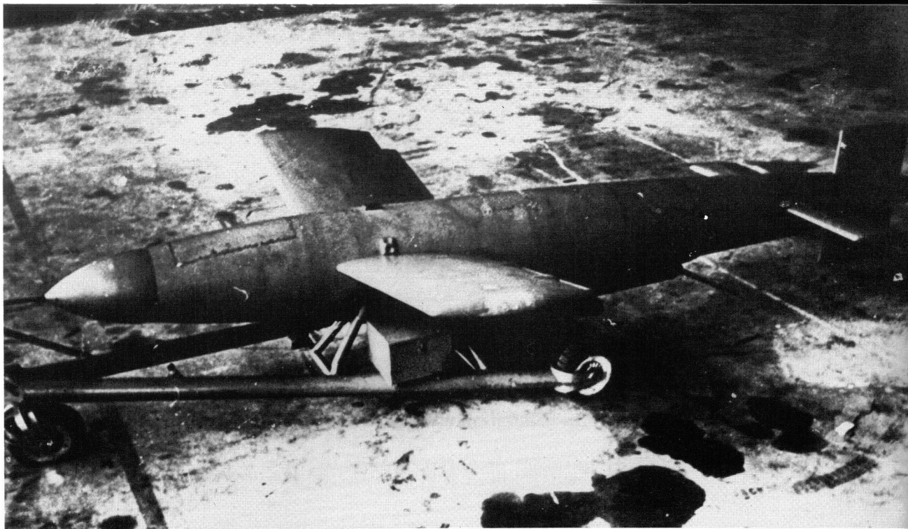
It was hoped that accuracy and range of the torpedo would be increased with the steerable Bv 143 over-water torpedo.
