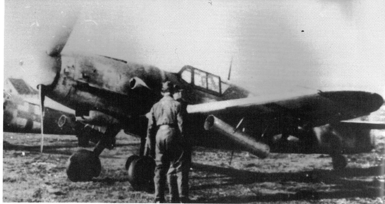
Above: A Messerschmitt Bf 109 G-6/R2 with firing tubes for the WGr. 21cm.
