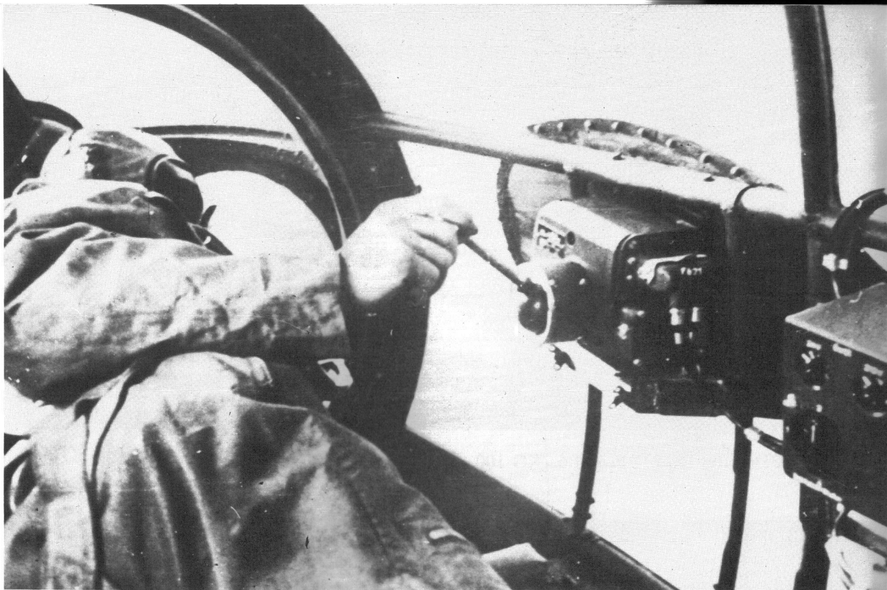
Above: The FuG 203 "Kehl III" guidance system in an He 111 H-18. Below: A Focke-Wulf Fw 200 C-4 with two Hs 293's.
