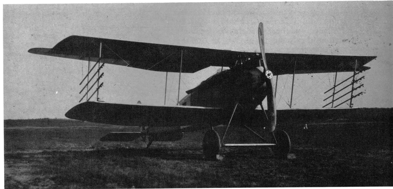
German Halberstadt D II single seater equipped with jury rigged incendiary rockets.
