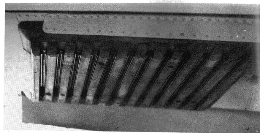
Above: Me 262 A-1a of the 9./JG7 with R4M firing tubes.
